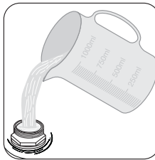
Only before filling with salt for the first time, fill the salt container with water.
